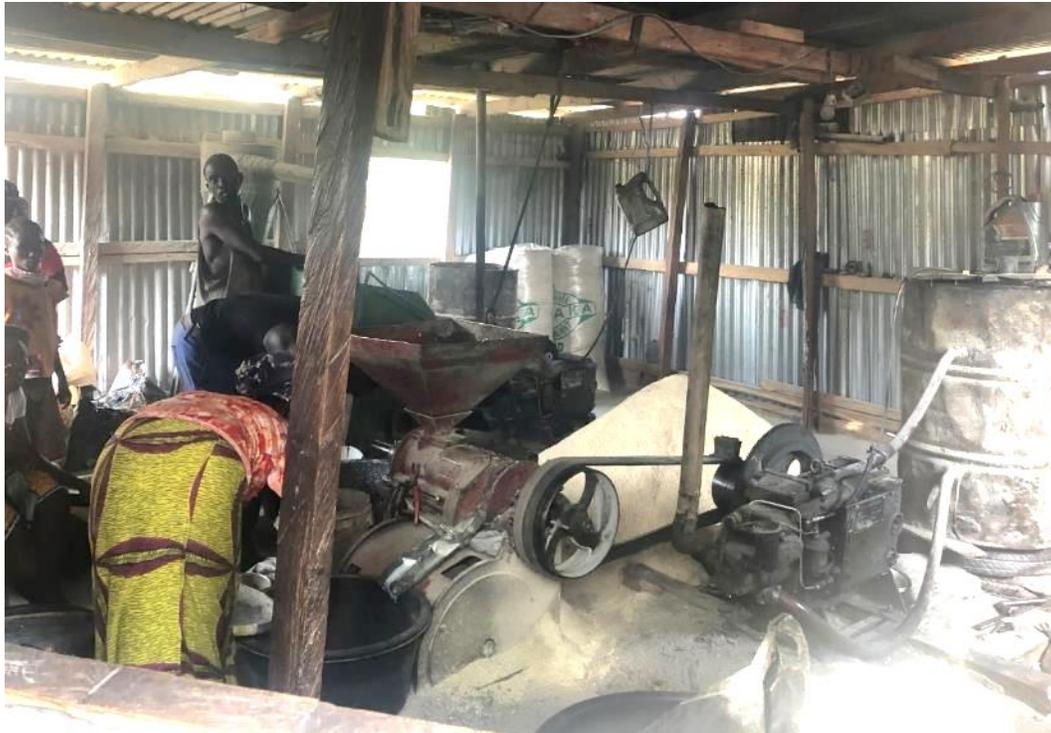
CAPTION: The grain mill operator at Kigbe, Nigeria uses diesel to power his mill.
